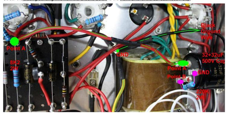
4. Solder a 100k/2W resistor and a 472J/630V capacitor together **in parallel** across the <u>Pin "Off" and Pin "On" of the Standby Switch</u>; Solder <u>one end of a red wire</u> onto the <u>Pin "On" of the Standby switch</u>, make sure you leave the red wire long enough to connect to the <u>Point B of the 32+32uF/500V capacitor</u>; See below:
